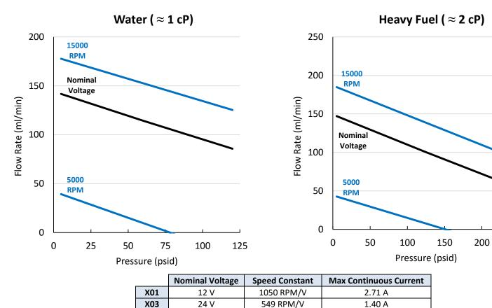
NOTES: Dashed lines indicate intermittent operation; speed constant may vary at higher pressures; RPM flow lines indicate performance at typical maximum and minimum speeds;
